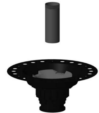
(1): REQUIRED WHEN NO ACCESS IS POSSIBLE UNDER THE BATH. ISLAND TUB DRAIN KIT INCLUDES ONE CONE-SHAPED DECK PLATE AND ONE 6 IN. (15 cm) THREADED TAILPIECE.
