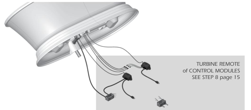
REMOTE MOUNTING OF TURBINE WITH ACCESS UNDER BATH
