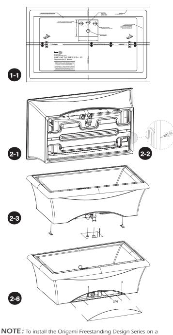
**NOTE :** To install the Origami Freestanding Design Series on a concrete slab with no place for the passage of the air inlet pipe to the bathtub: drill a hole 1 <sup>5/8</sup> inches in diameter in the skirt. IMPORTANT: drill the hole 1 <sup>1/2</sup> inches above floor level and protect the bathtub with a piece of wood placed behind the location to be drilled.
