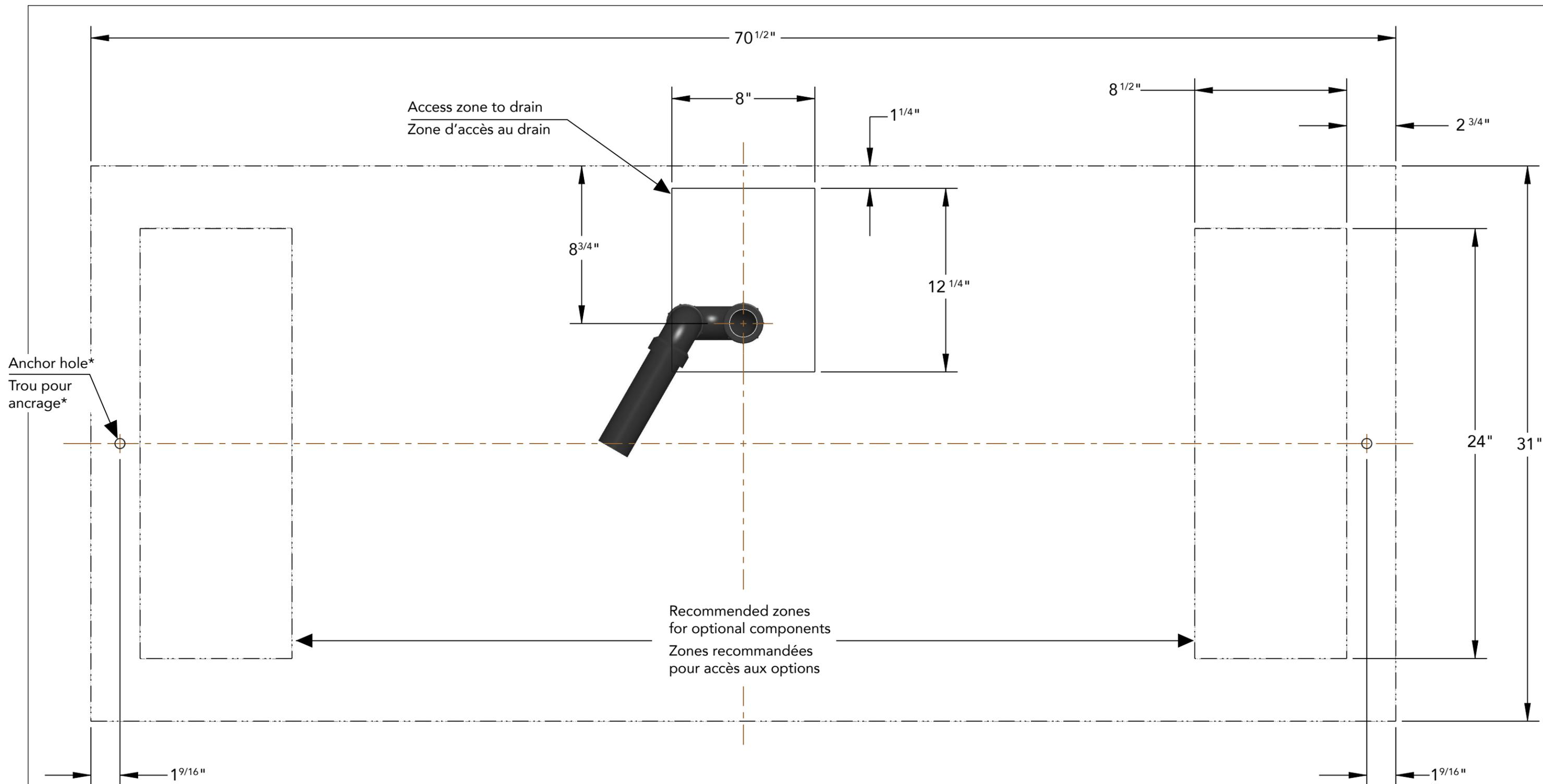
**(\*) WARNING: Always use the real measurements** to position of openings on the tub and to align the anchors to the floor.
