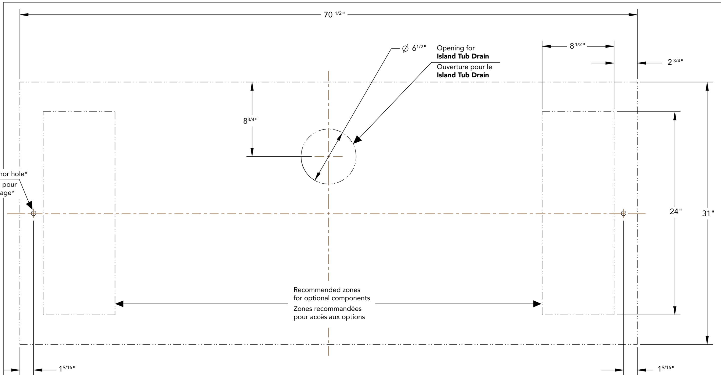
**(\*) WARNING: Always use the real measurements** to position of openings on the tub and to align the anchors to the floor.
