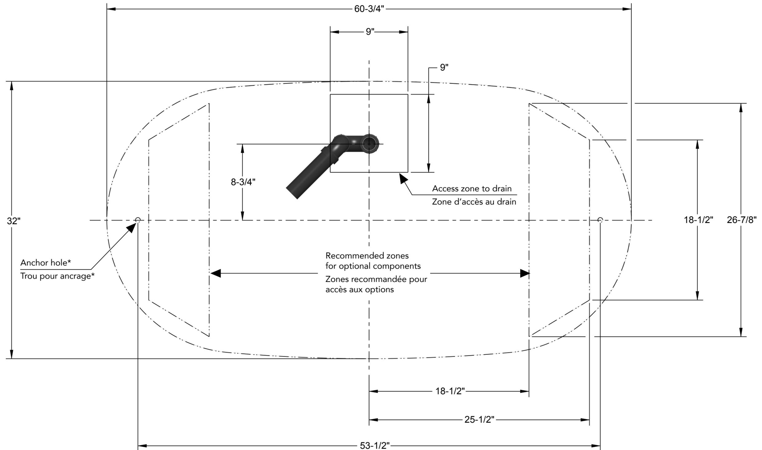
(\*) **WARNING: Always use the real measurements** to position of openings on the tub and to align the anchors to the floor.
